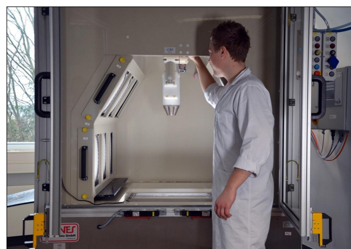
Centrifuge-electrospinning: Cutting-edge technology for the up-scaled production of nano- to submicron biopolymer fiber mats.
